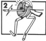
2 Place flat surface into loop of clip
