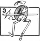
3 Twist insert around loop of clip
