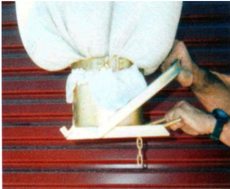
Fig. 1 Davis Bag Mate attached to the bladder of bulk bag.
