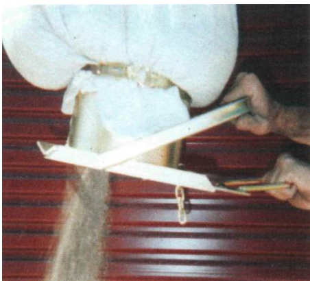
Fig 3. Davis Bag Mate sliding shutter is opened for controlled release of grain.
